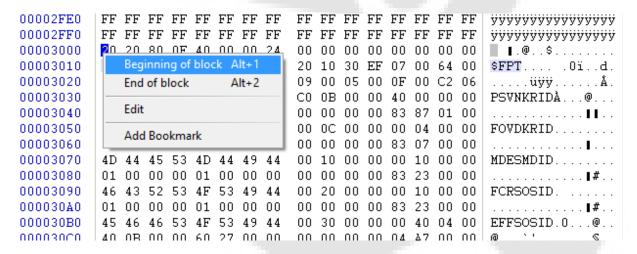
Next Ctrl+B, and then saved as new file. use the programmer to write the BIOS chip.
